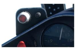
In case of issues with lights, you can use the auditory check button. Once pressed, a continuous sound will be emitted if landing gear is down and locked.
