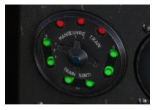
A light above main panel will blink when one of the engines is below 15,000 RPM and the landing gear is not down.
