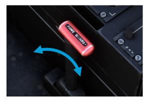
4. Stop pumping once the three landing gear lights are green.
