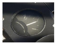
When defrost is selected, air is directed upon the windshield. In addition, defrost handle on the main panel allows to spurt alcohol on the front glass to help defrosting (action is not simulated).
