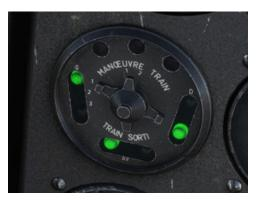
It is not possible to retract the landing gear using emergency circuit.
