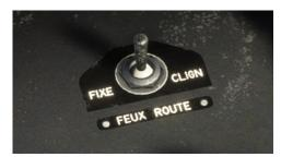
As we have to manage three distinct position, keyboard input cannot be taken into account. You need to use the switch on the left console to turn on or off the navigation lights.
