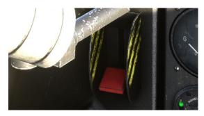
2. Click on the button to use secondary hydraulic circuit.
