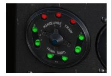
A light above main panel will blink when one of the engines is below 15,000 RPM and the landing gear is not down.
