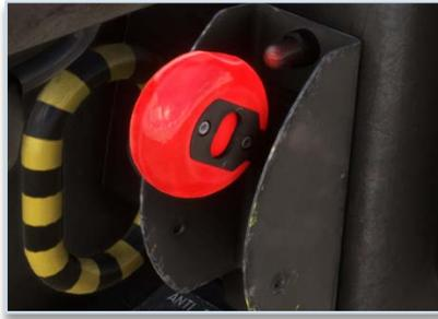
Fire alarms are triggered if a fire is detected in zone 1 or zone 2 of the engines, they are described [here](#).
