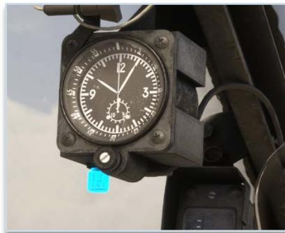
This light is dedicated to the instruments located above the panel: clock, standby compass, angle of attack indicator and accelerometer.
