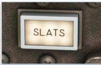
In manual mode, slats are controlled by a switch on left console (extended – neutral – retracted).
