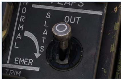
Above 500 knots, slats cannot be extended any more, and can only be retracted.
