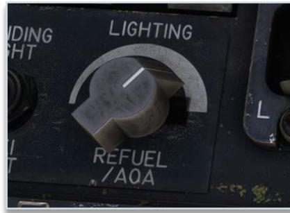
By default, refueling lights cannot be used if refueling probe is retracted. A switch behind a hood is used to force refueling lights even in that case:
