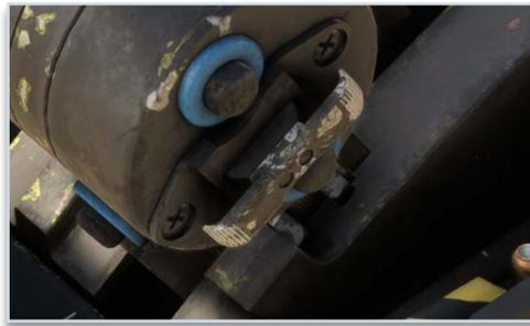
The airbrakes remain hydraulically locked in any intermediate position or at full extension. The full extension or retraction time on the ground is approximately 3 seconds.
