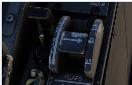
An emergency "override" switch allows flap extension even in case of a slat deployment failure.
