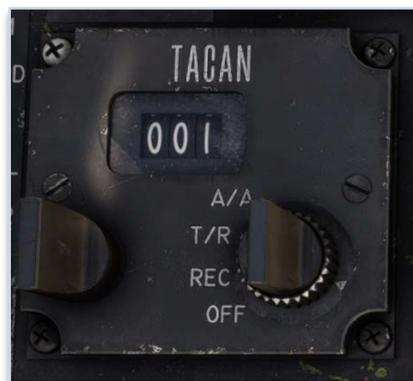
Switch between X/Y modes can be done by clicking on the channel window frame, or from the EFB tablet (second tab).
