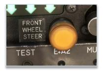
When the aircraft is empty, with steering engaged, the minimum turning radius is 7.10 m.
