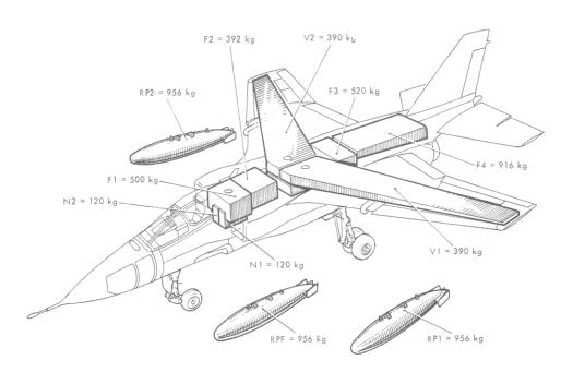
N1 and N2 tanks are connected to left and right engine (respectively). They are the only tanks having a flexible structure.
