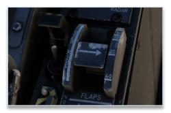
An emergency "override" switch allows flap extension even in case of a slat deployment failure.
