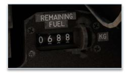
A button on the EFB allows to set the totalizer automatically.
