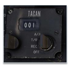
Switch between X/Y modes can be done by clicking on the channel window frame, or from the EFB tablet (second tab).
