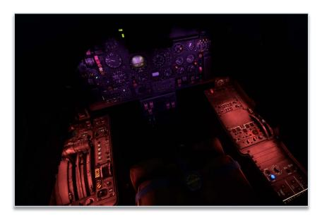
Panel and console lights can be set at different intensities with three knobs above right console. For instruments panel, red lights or UV lights (or a mix of both) can be chosen.
