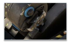
The airbrakes remain hydraulically locked in any intermediate position or at full extension. The full extension or retraction time on the ground is approximately 3 seconds.
