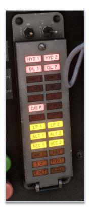
Any warning alarm will also trigger master warning alarm (blinking light and alert sound).
