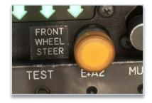
When the aircraft is empty, with steering engaged, the minimum turning radius is 7.10 m.
