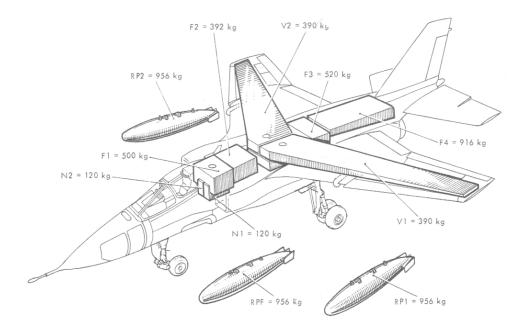
N1 and N2 tanks are connected to left and right engine (respectively). They are the only tanks having a flexible structure. F2 and F3 tanks are directly connected. Transfer between other tanks is managed with the help of several electro-valves. All tanks (except N1, N2, F2/F3 and F4 which enclose transfer pumps) are pressurized with air taken from the engines.
