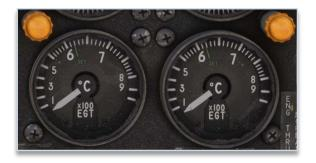
EGT amplifier switches can have an impact on the temperatures reached. On normal position (ON), it enables automatic regulation of the limit temperatures, and restricts the maximum speed of the low-pressure spool (by reducing fuel flow).
