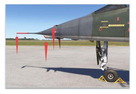
By walking around the aircraft, you can inspect various parts (struts, rudder, elevator, etc) and check their condition before flying. Each part to inspect or remove is indicated by a circled dot.
