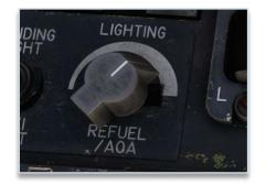
By default, refueling lights cannot be used if refueling probe is retracted. A switch behind a hood is used to force refueling lights even in that case:
