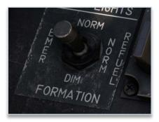
A knob allows to set refueling lights intensity. This same knob also commands intensity of AoA indicator light.
