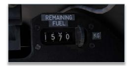
A button on the EFB allows to set the totalizer automatically.
