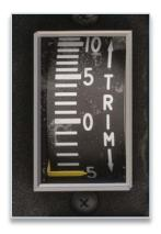
Rudder trim is managed with a switch on the left console, and a small indicator indicated:
