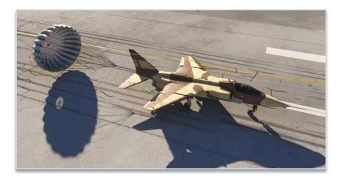
Once the aircraft has been slowed, pushing parachute handle will release it. The object will stay where it has been released.
