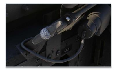
The chute will be deployed only once landing gear is in contact with the ground, and will drastically brake the aircraft thanks to its aerodynamic drag.
