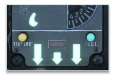
Landing gear should not be extended above 250 knots to avoid any damage.
