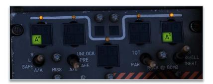
Only one missile can be launched at a time, and you need to set the air/air missile safety switch to the desired position ("L" for left, "R" for right).
