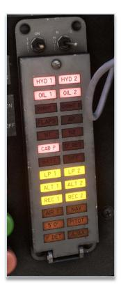
Any warning alarm will also trigger master warning alarm (blinking light and alert sound).
