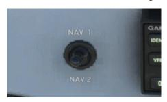
NAV 1 frequency is set from the GPS and NAV 2 frequency from the secondary radio unit.
