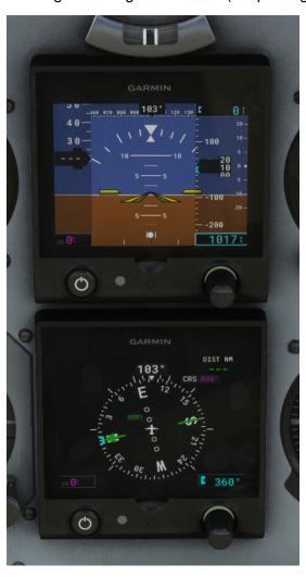
You can switch between VLOC and GPS mode from the GPS unit. In VLOC mode, NAV 1 source will be used.
