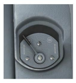
An inverted flight feeder tank which contains 2.5 litres allows a limited time of inverted flight. Rollover valves installed in each tank limit fuel waste through air vents during inverted flying. After approximately two minutes of inverted flying, fuel feeding will stop, resulting in engine shutdown.
