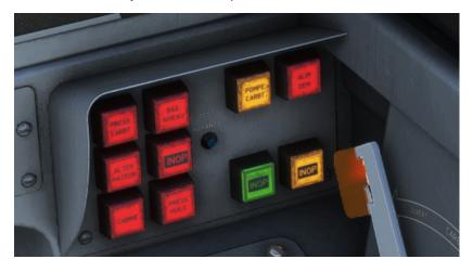
A button allows to test correct lighting of each alarm.
