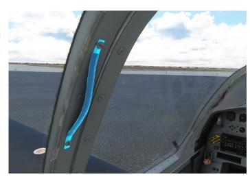
Front canopy locking against the windshield is performed by two side catches in which enters the windshield locking pins. The rear canopy locking against the front canopy is identical.
