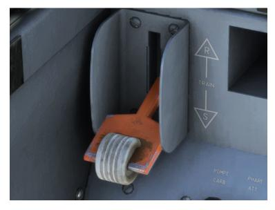
Then, you need to pull emergency gear lever to let the landing gear going down.
