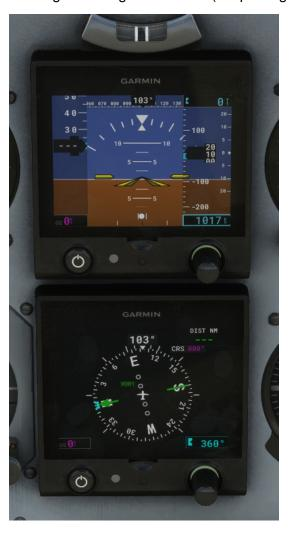
You can switch between VLOC and GPS mode from the GPS unit. In VLOC mode, NAV 1 source will be used.
