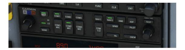
It features two double knobs to set pilot/copilot intercom volume and squelch level, and the following buttons:
