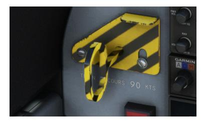
Once emergency handle is pulled, landing gear cannot be manipulated anymore until hydraulic pressure is available again.
