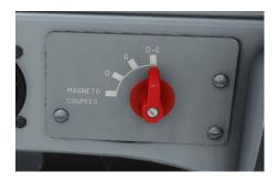
Ignition is performed through a dual magneto, which provides spark plugs with a high-voltage double ignition (two spark plugs per cylinder). Ignition order is 1-4-5-2-3-6.
