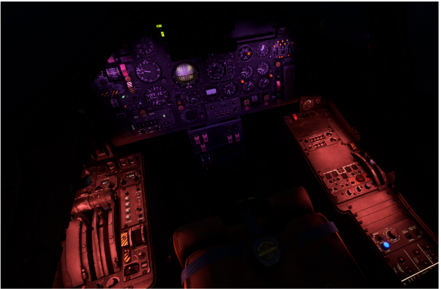
Panel and console lights can be set at different intensities with three knobs above right console. For instruments panel, red lights or UV lights (or a mix of both) can be chosen.
