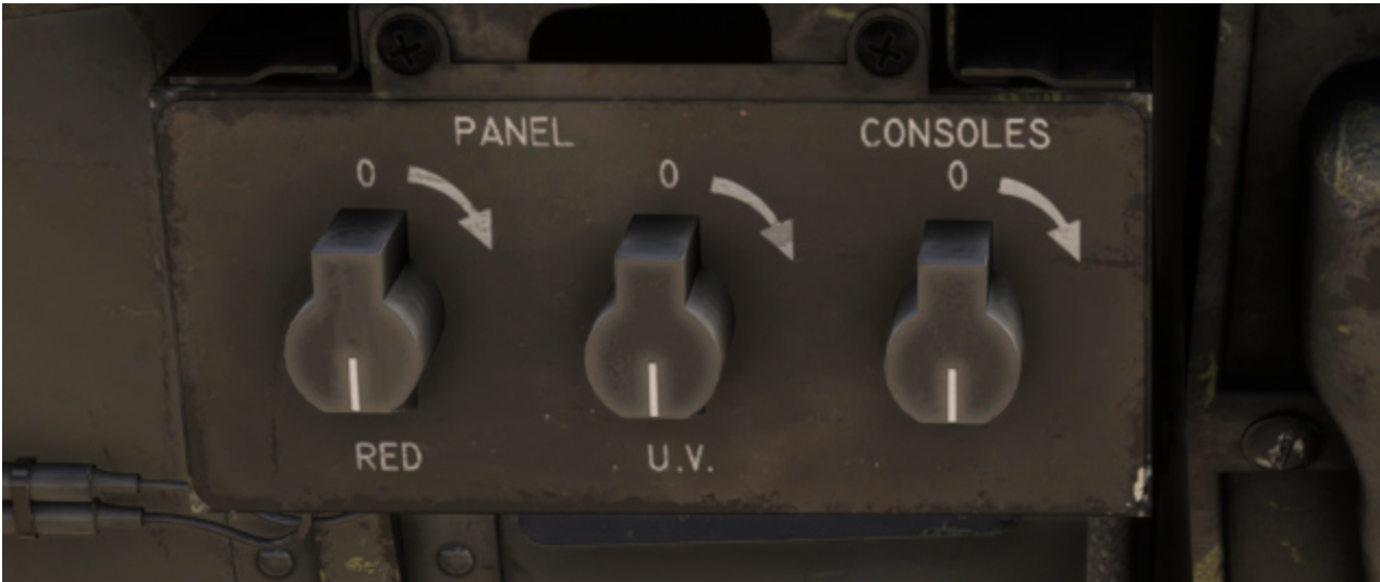
Integrated lights can be set at different intensities, independently for left and right side of the cockpit (left console):
