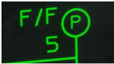
Booster pump operating
