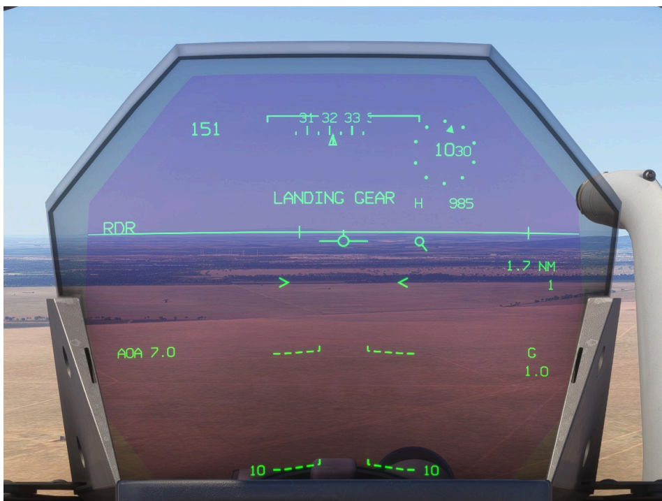
Landing gear alert displayed on HUD
