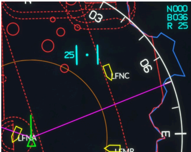
Cursor located 25 nm away on a bearing of 36°
