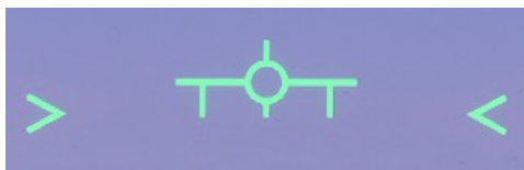
VVI with the landing gear down and locked
