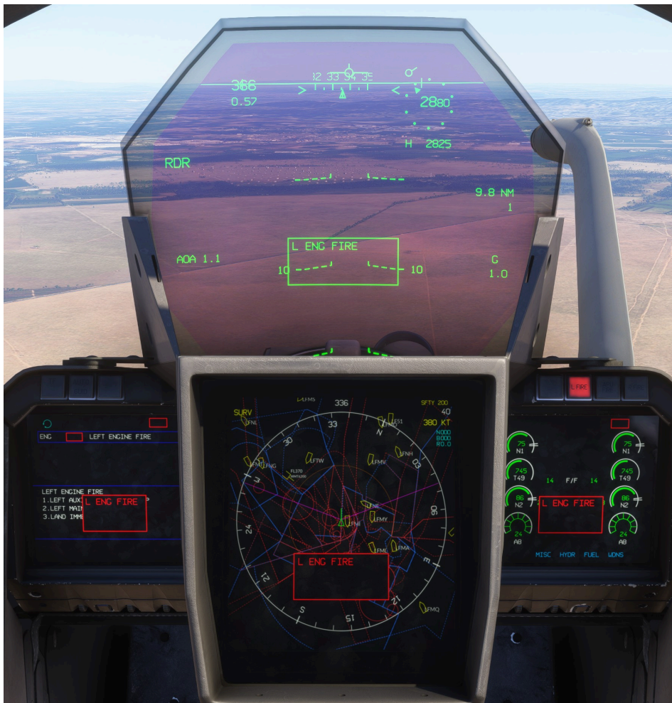
Red alarm displayed on main avionics screens
