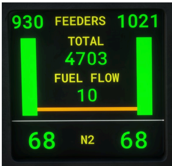
Feed tanks crossfeed valve open
