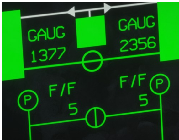
Feed tank crossfeed valve open, low-pressure crossfeed valve closed
