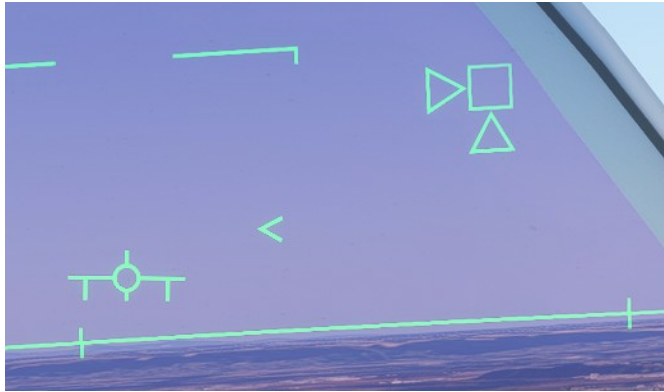
Guidance indicating a climb and a correction to the right to rejoin the approach path
