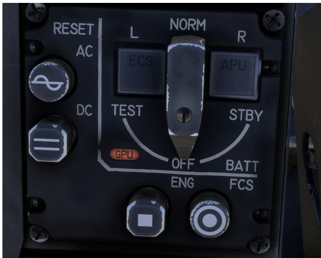
Indicator confirming that GPU is providing electricity
