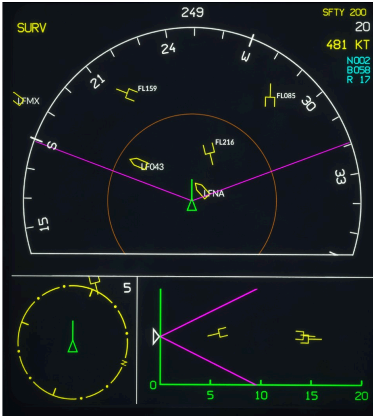
HCD with the expanded view and A2D view displayed
