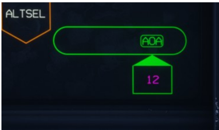
Autothrottle enabled in AOA mode with a target of 12 degrees
