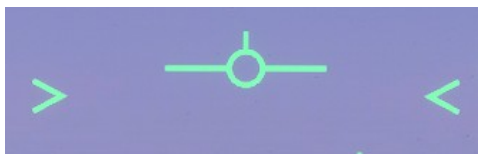
VVI with the landing gear retracted
