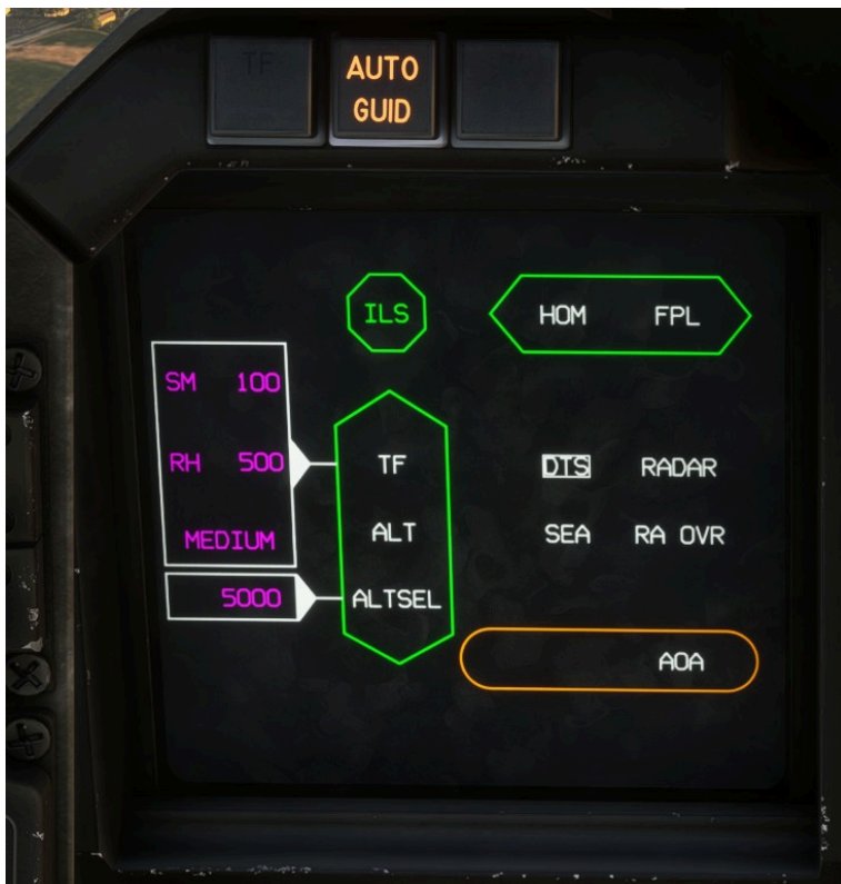
LD AP page with ILS approach mode active, as confirmed by the AUTO GUID indicator
