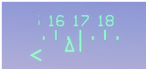
Heading ribbon showing a five-degree deviation
