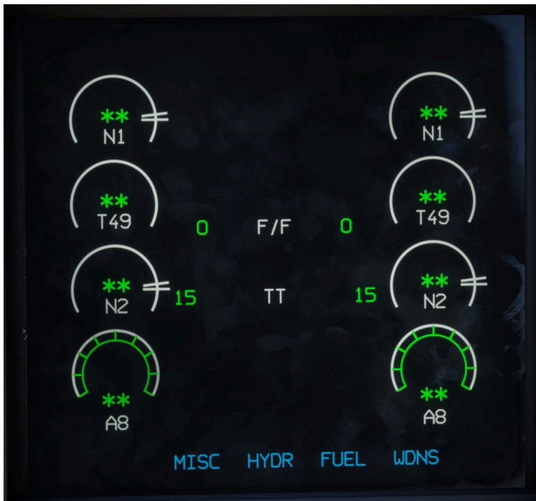
Display with the engine control units unpowered
